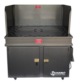
Dynamo Grind Series tables feature a ¼" heavy-duty steel top, 3-sided moveable spark shield, flame-retardant push-button pulse cleaning cartridge filtration and an ember-catching water tray. These tables are using for welding and all types of metal applications (grinding, welding, cutting, polishing, etc.). These tables cannot be used for any type of magnesium or aluminum application.
